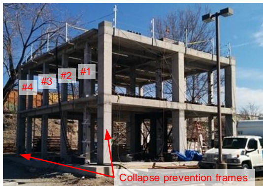
(a) Front view of the four testing frames, enveloped by two collapse-prevention frames
