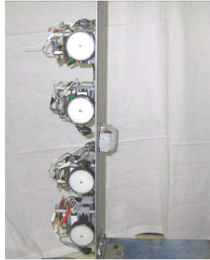
Figure 9. Damage Scenario I – an extra mass block and two mobile sensing nodes, one node allocated at location A1, and the other node at A2 (locations A1 and A2 are as shown in Figure 5b).
