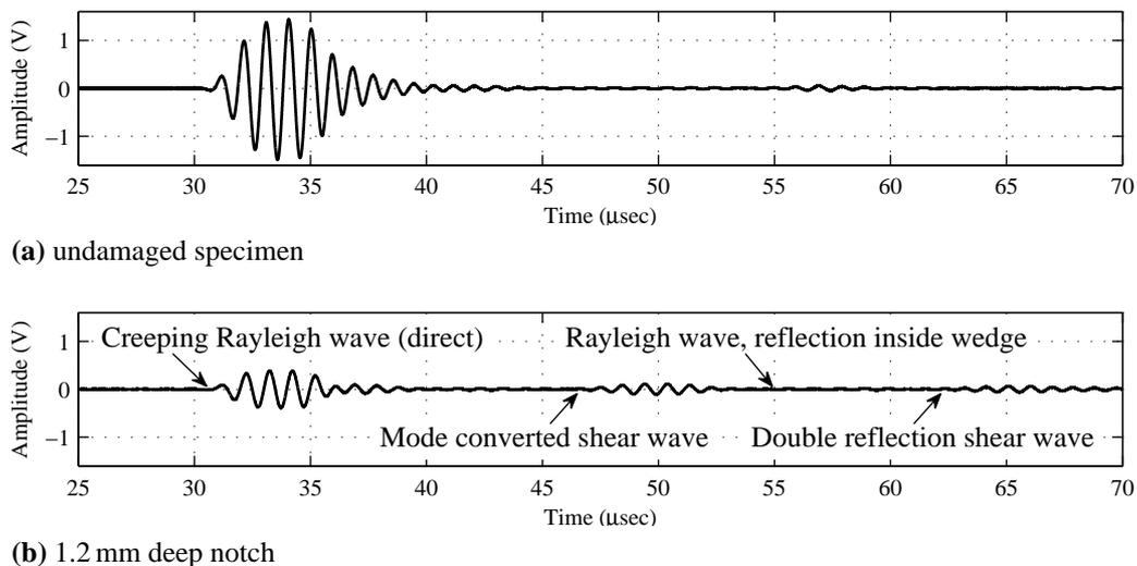
**FIGURE 3.** Ultrasonic measurement signals in the time domain for different notch depths, taken with commercial ultrasonic equipment.
