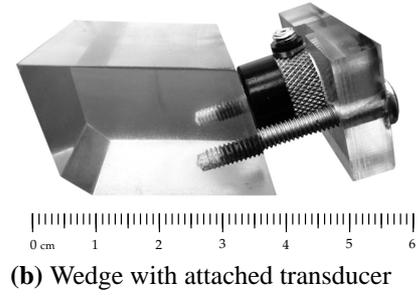
**FIGURE 2.** Generation of Rayleigh waves using a contact transducer and a coupling wedge.
