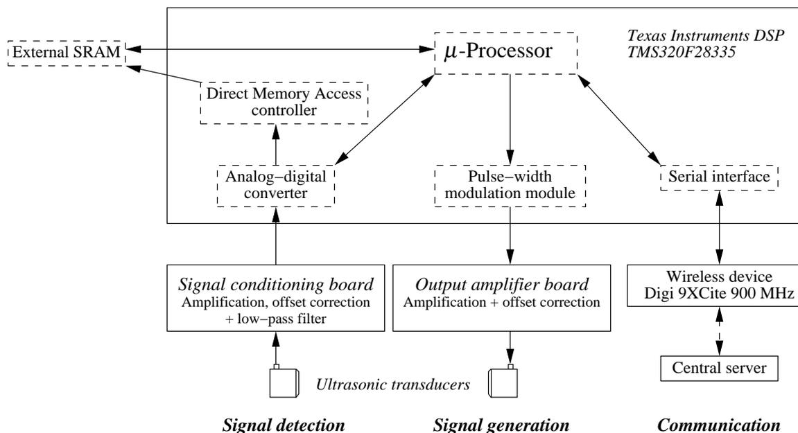
**FIGURE 1.** Functions and parts of the device. The signal path to the left illustrates the signal detection, the signal path in the middle the signal generation. The wireless device to the right in the figure enables communication with a central server.
