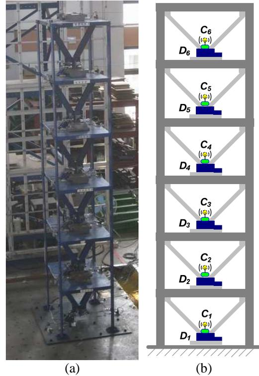
Figure 2. Six-story structure for control experiments: (a) picture of the structure on the shake table; (b) schematic of the setup,  $C_i$  – wireless sensing/control unit connected with a position sensor measuring inter-story drift;  $D_i$  – magnetorheological (MR) damper.
