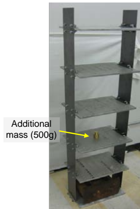
Figure 13. Damage scenario I – A 500g additional mass is attached on the 2nd floor
