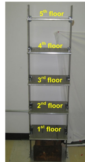
Figure 8. A five-story shear-building structure
