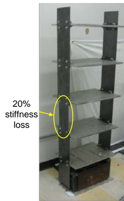
Figure 16. Damage scenario II - 20% stiffness loss is introduced to the section of one column between 2nd and 3rd floors
