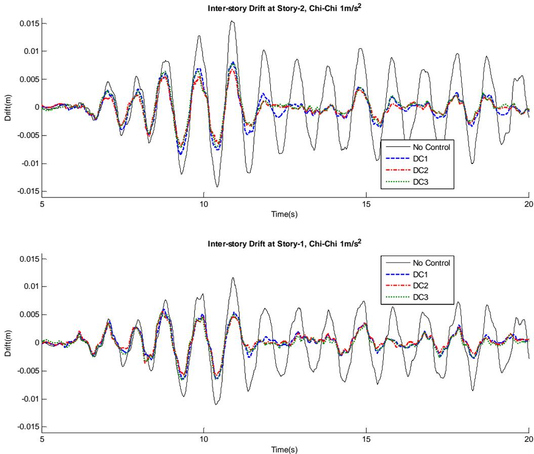
Fig. 6. Experimental inter-story drift histories from different system architectures for the Chi-Chi excitation scaled to a peak acceleration of  $1\text{m/s}^2$  (different degrees of decentralization as illustrated in Fig. 4).
