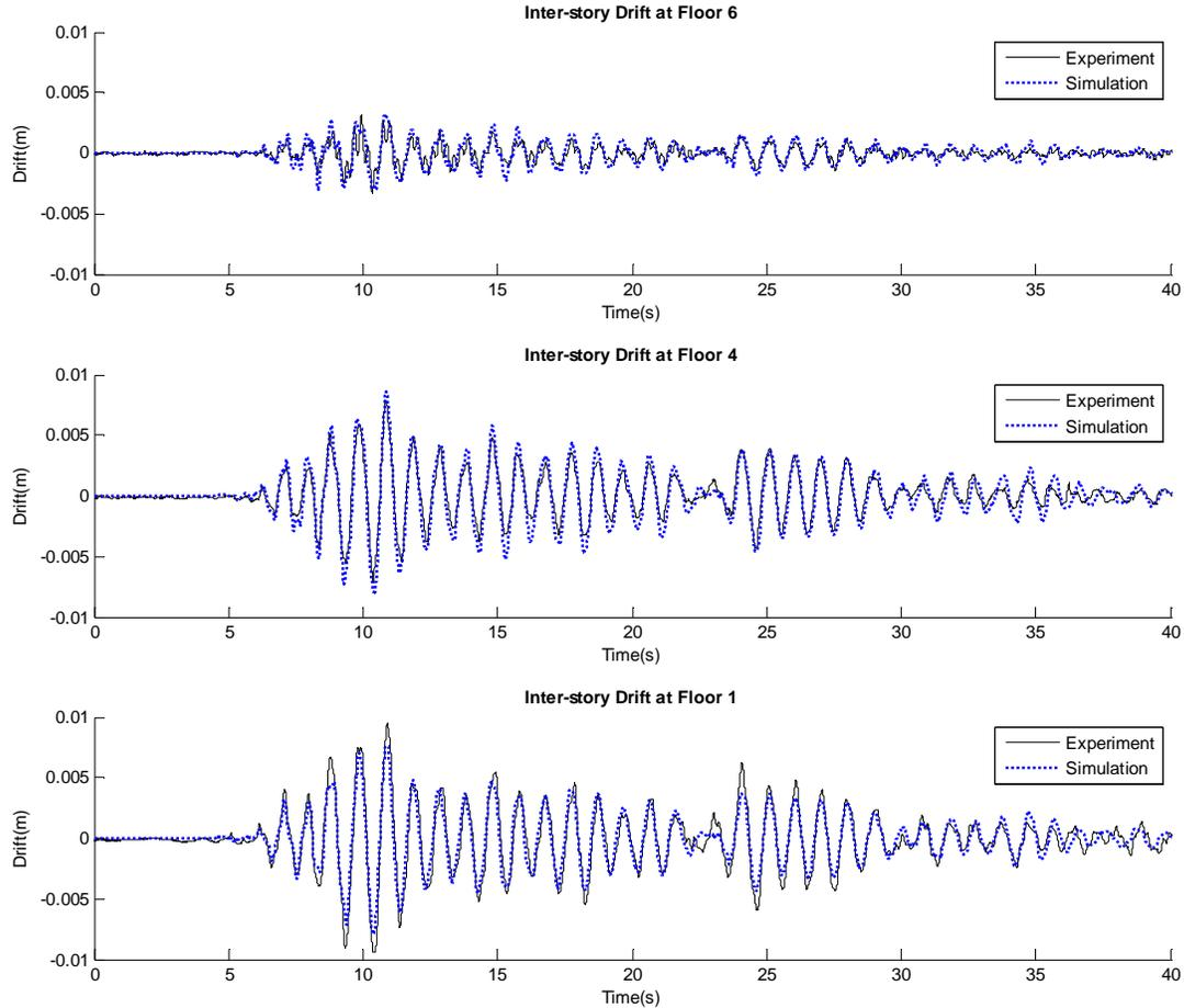
Fig. 3. Experimental and simulated inter-story drifts for a Chi-Chi (TCU-076 Station) earthquake excitation with the peak acceleration scaled to  $1\text{m/s}^2$ ; command voltages to all six dampers are fixed at  $0\text{V}$ .
