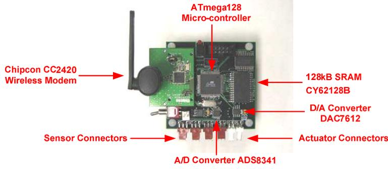
Fig. 1. Narada wireless sensing/actuation unit designed by Swartz and Lynch [16].
