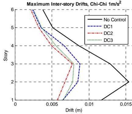
Fig. 5. Experimental peak inter-story drift results of different system architectures for the Chi-Chi excitation scaled to a peak acceleration of  $1\text{m/s}^2$  (different degrees of decentralization as illustrated in Fig. 4).
