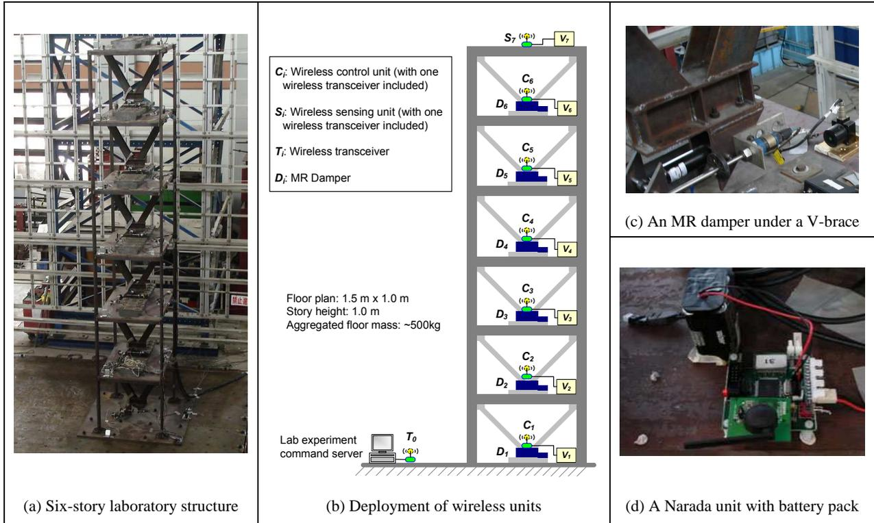
Fig. 2. Experimental setup for wireless feedback control of a six-story structure.
