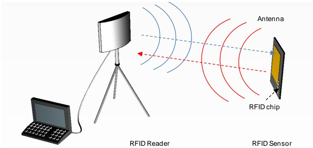
Fig. 1. Conceptual illustration of RFID reader and sensor
