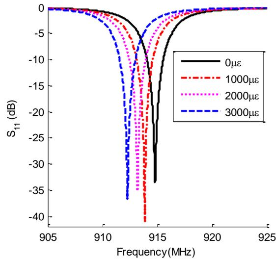
(a)  $S_{11}$  parameters under strain transfer
