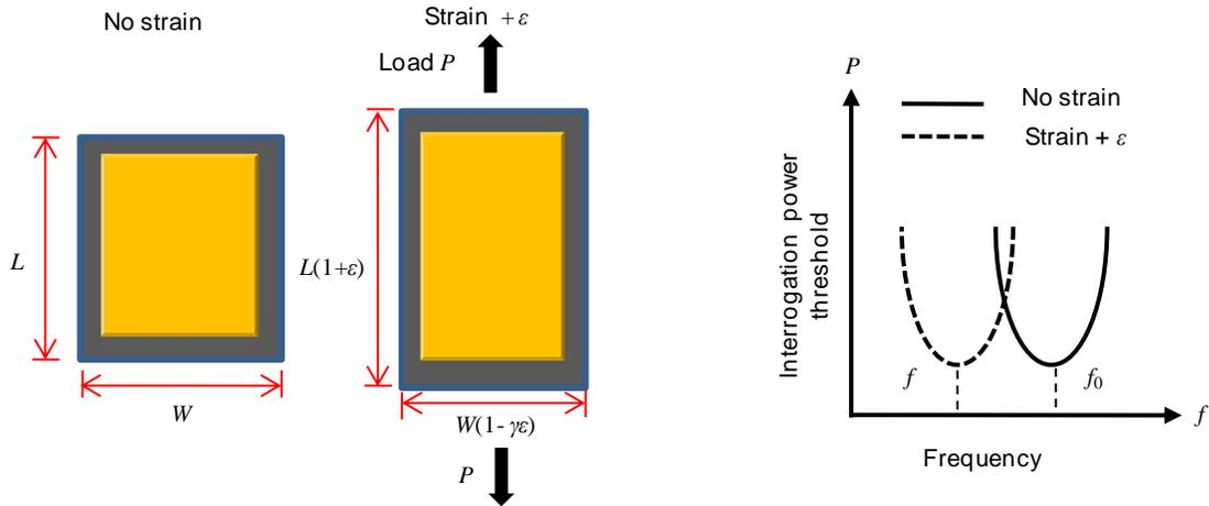
(a) Antenna deformation in the longitudinal direction (b) Illustration of interrogation power threshold measurement
