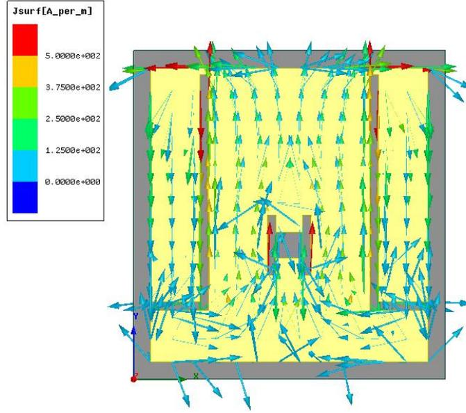
Fig. 8. Surface current density vector of the slotted patched antenna sensor simulated in Ansoft HFSS
