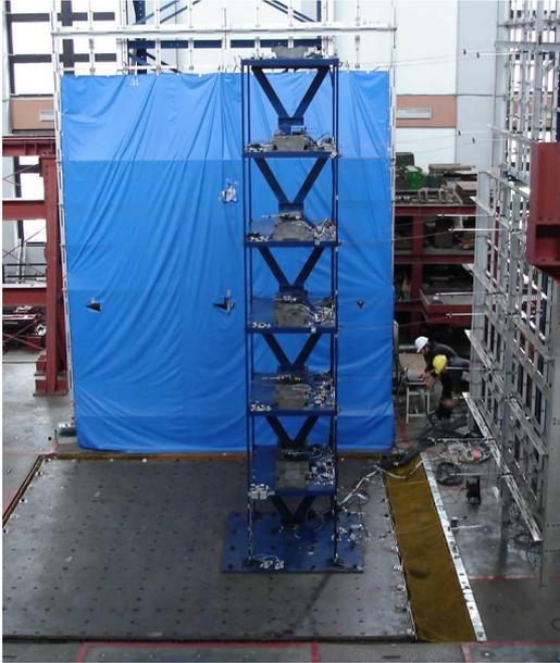
Figure 3 Six-story test structure mounted to the 25 m<sup>2</sup> shaking table at the National Center for Research on Earthquake Engineering (NCEE), Taipei, Taiwan
