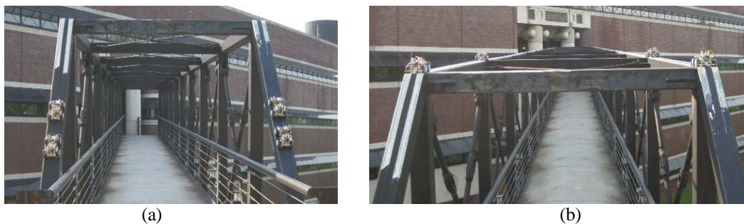
Figure 2. Pictures of four mobile sensing nodes navigating on the space frame bridge: (a) The mobile sensing nodes start from the incline members; (b) The mobile sensing nodes arrive at the 1 st measurement configuration.
