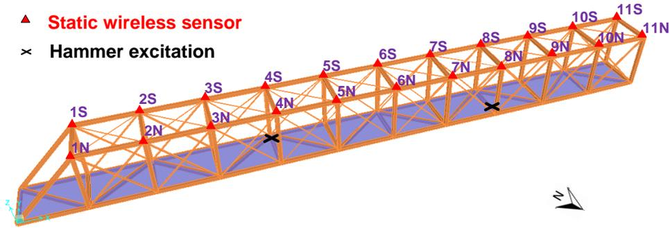
Fig. 3. Experimental setup for the testing with static wireless sensors.
