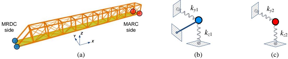
Fig. 8. FE model for the steel bridge: (a) 3D view of the bridge model; (b) support condition at MRDC side for model updating; (c) support condition at MARC side for model updating.
