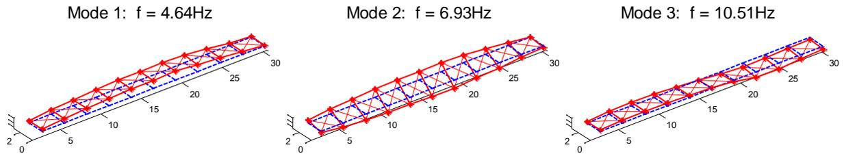
Fig. 7. First three mode shapes of the bridge extracted from static sensor data with hammer impact excitation.
