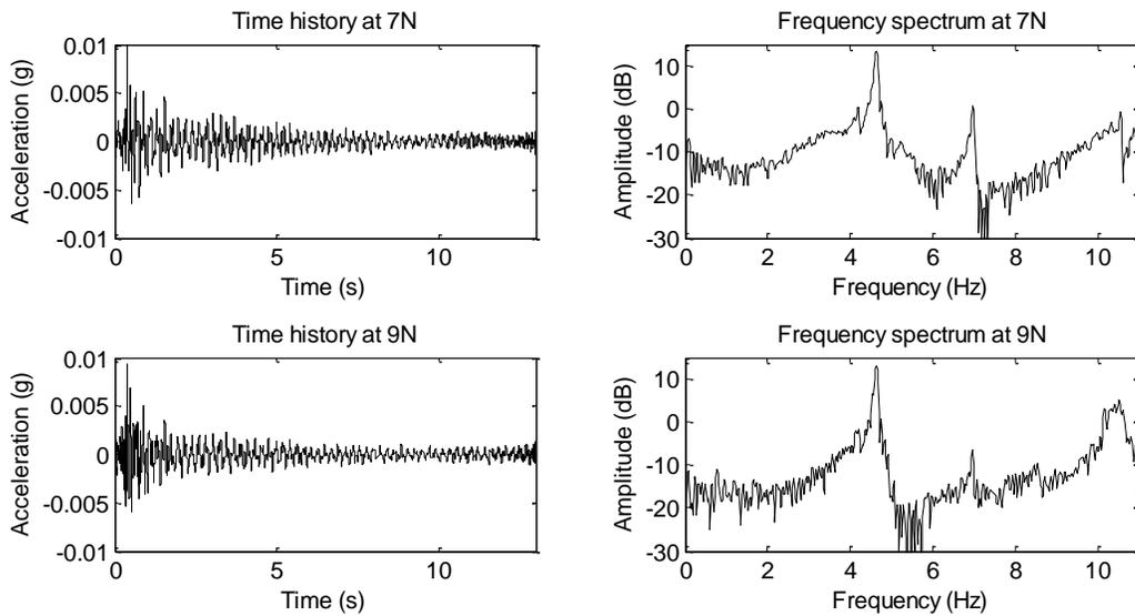
Fig. 4. Example vibration records and corresponding frequency spectra recorded by mobile sensors when hammer impact is applied on the floor below location 8N.
