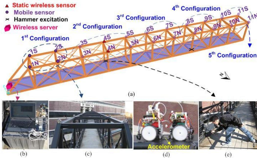
Fig. 2. Experimental setup for mobile sensor testing: (a) 3D illustration of five measurement configurations for the MSNs; (b) a laptop as the wireless server; (c) four MSNs deployed at the 1<sup>st</sup> configuration; (d) an MSN attaches an accelerometer onto the structural surface; (e) a hammer impact is being applied.
