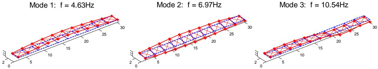
Fig. 6. First three mode shapes of the bridge extracted from mobile sensing data with hammer impact excitation.
