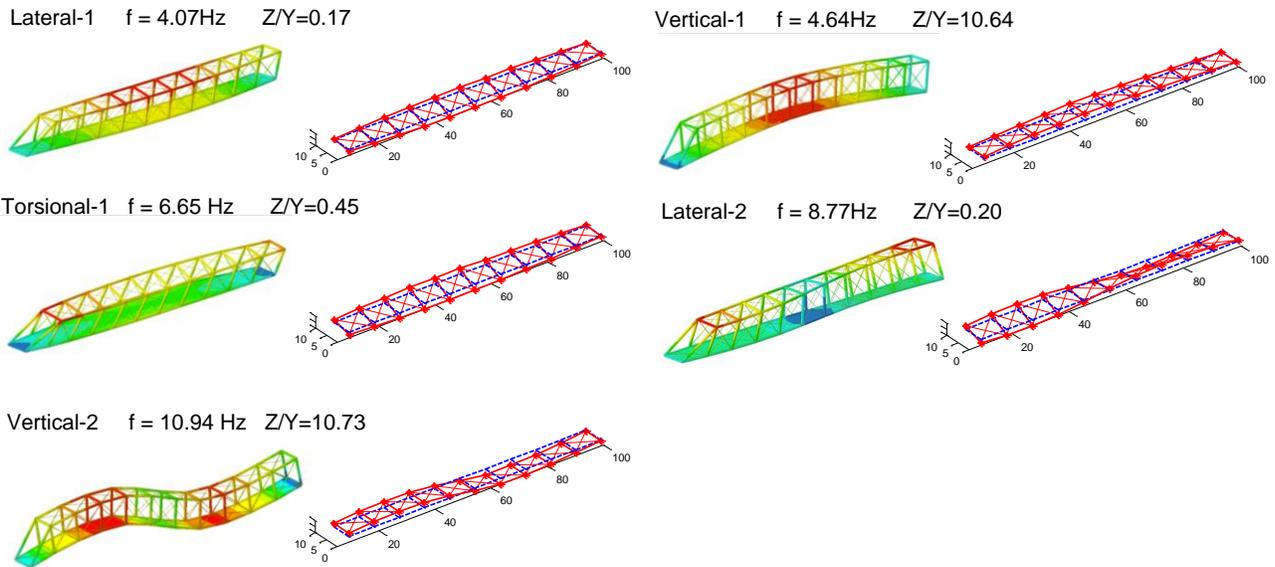
Fig. 9. First five mode shapes of the FE model.
