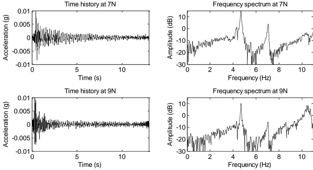
Fig. 5. Example vibration records and corresponding frequency spectra recorded by static sensors when hammer impact is applied on the floor below location 8N.
