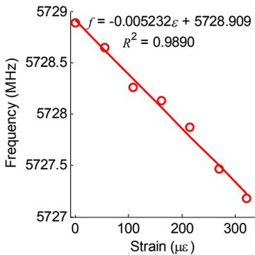
(b) Resonance frequency change versus strain
