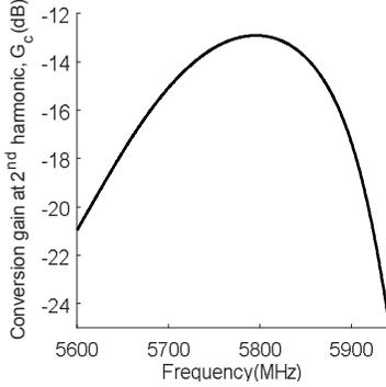
(b) Simulated conversion gain at the 2<sup>nd</sup> harmonic,  $G_c$  at -10 dBm input power
