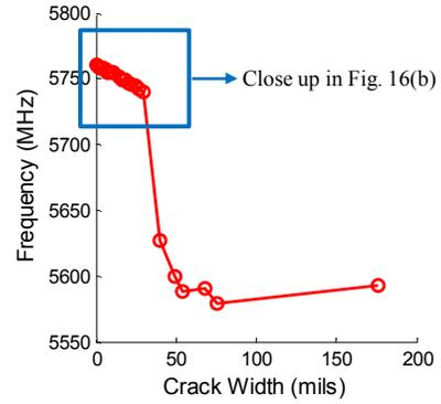
(a) Resonance frequency change during crack growth
