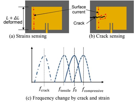
Fig. 2. Strain/Crack simulation mechanism of a patch antenna sensor
