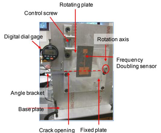
Fig. 12 Emulated crack device
