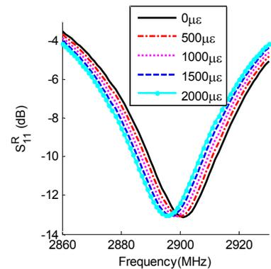
(b) Simulated  $S_{11}^R$  parameter under strain
