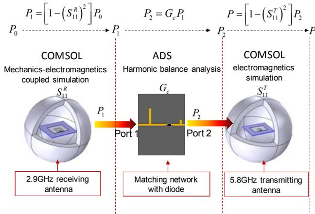
Fig. 6. Flow chart of the multi-physics coupled simulation for the entire sensor
