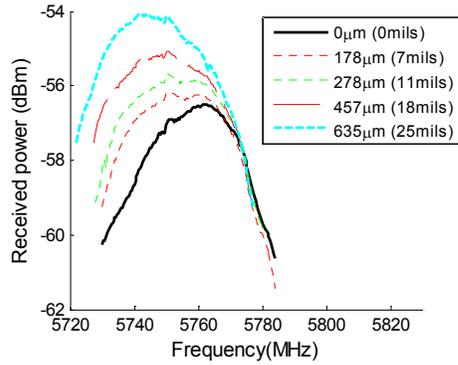
(a) Crack size from 0 to 25 mils
