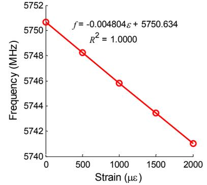
(b) Resonance frequency versus strain curve
