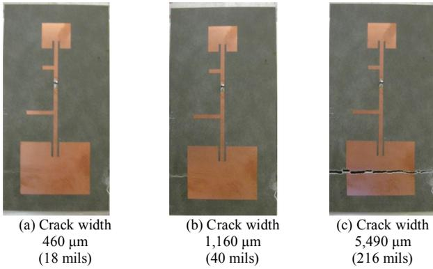
Fig. 13. Photos of deformed antenna sensor at different crack opening sizes
