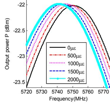
(a) Output power with different strain level
