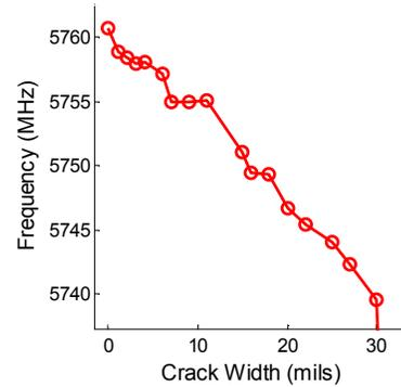
(b) Resonance frequency change during crack growth (closed-up view to 0-30mils)
