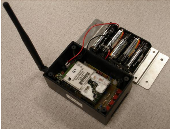
Figure 4: WiMMS wireless sensor node
