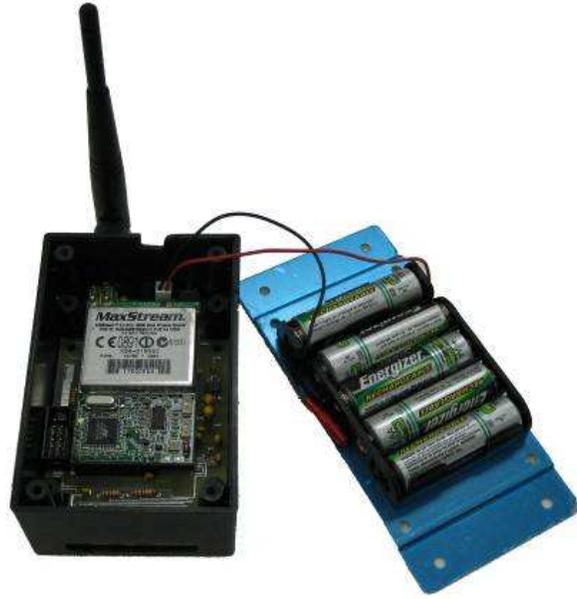
Figure 3. Wireless sensing prototype
