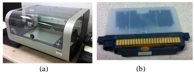
Fig. 5. Printing equipment. (a) Dimatix Materials printer; (b) Cartridge.
