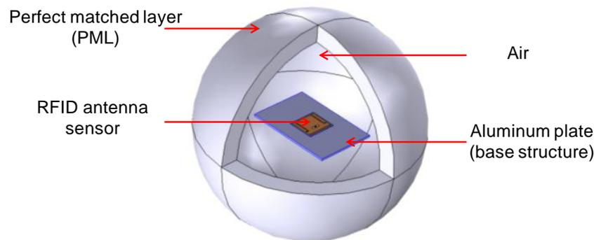
Figure 2. Multi-physics simulation model using COMSOL
