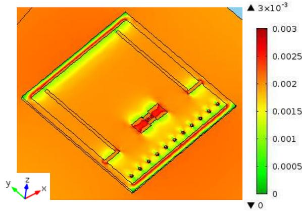
Figure 3. Strain distribution  $\epsilon_y$  of the aluminum plate and the antenna sensor
