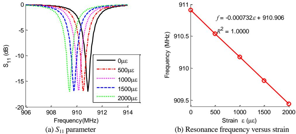
Figure 4. Strain simulation results of the antenna sensor generated by COMSOL
