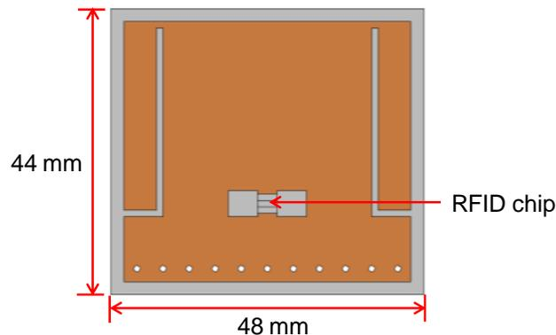
Figure 1. Design drawing of the slotted patch antenna sensor (top view)
