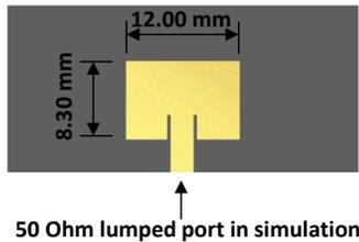
(a) Dimensions of the 11.6 GHz transmitting antenna
