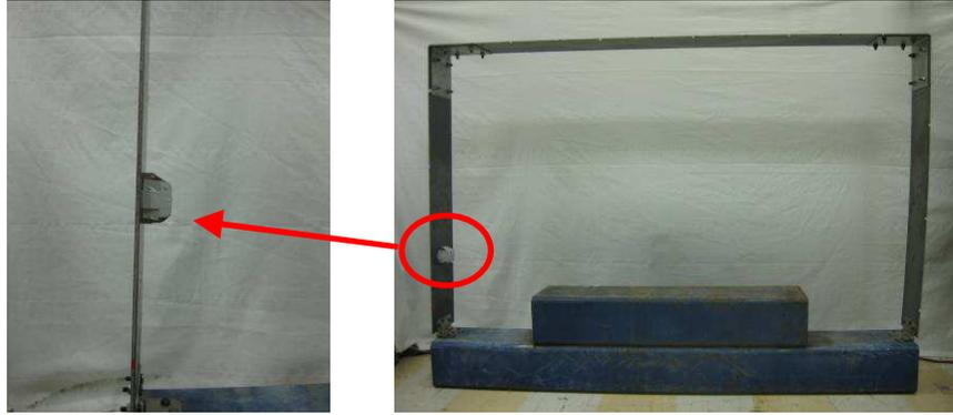
**Figure 4. Damage Scenario I - an extra mass block mounted between locations A1 and A2.**
