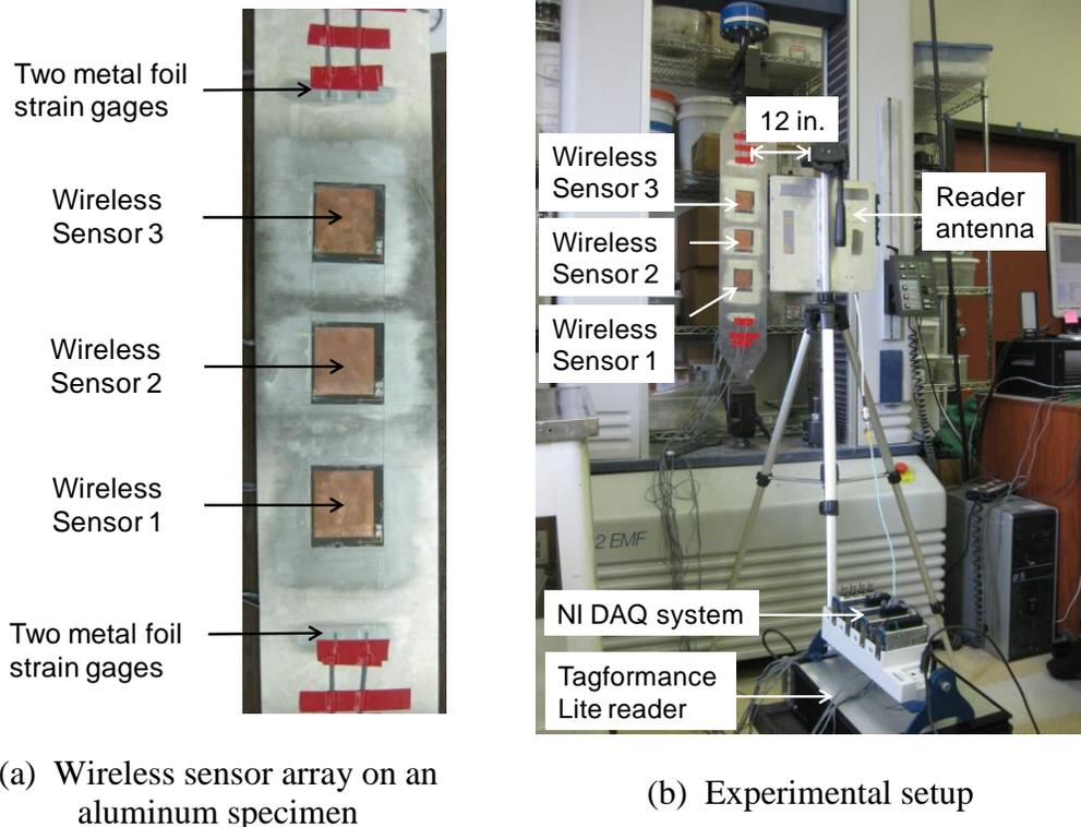
Fig. 4. Experimental setup for the tensile test with a wireless sensor array
