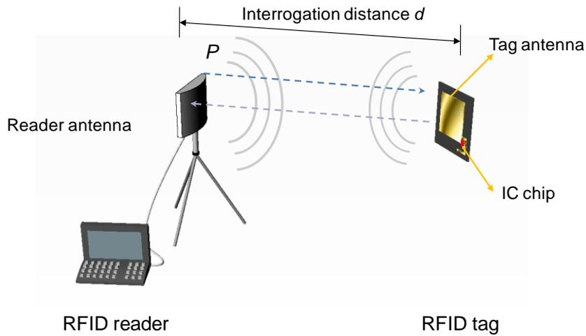
Fig. 1. Power transmission and backscattering in a passive RFID tag-reader system for wireless strain sensing
