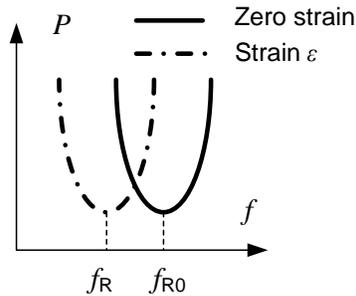
Fig. 3. Conceptual illustration of the resonance frequency shift due to strain
