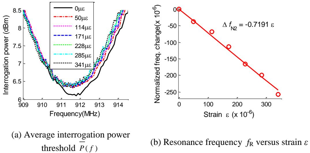
Fig. 6. Tensile testing results for Sensor 2
