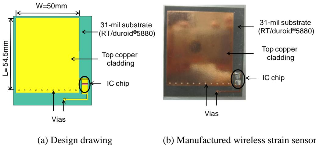
Fig. 2. RFID tag as wireless strain sensor
