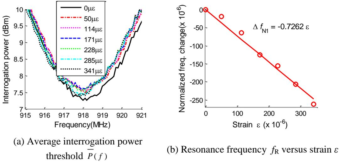
Fig. 5. Tensile testing results for Sensor 1
