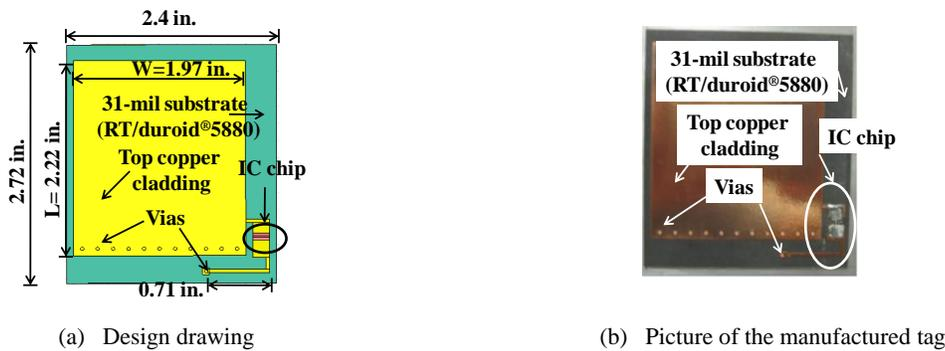
Fig. 2. RFID tag as wireless strain sensor (Prototype A)
