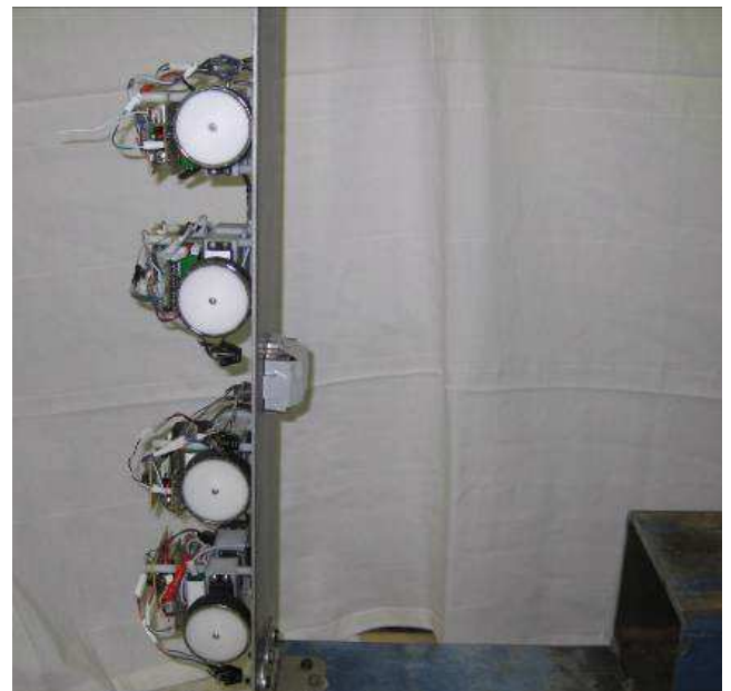
Figure 4. Additional mass block and two mobile sensing nodes, one node allocated at location A1, and the other node at A2 (locations A1 and A2 are as shown in Figure 3).
