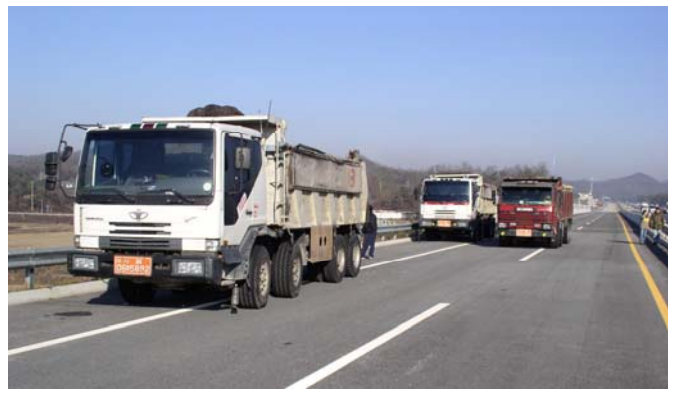
Figure 3. Three trucks (15, 30, and 40 tons) are used to induce vibrations in the Geumdang Bridge
