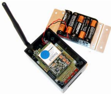
Figure 1. Wireless sensor deployed in the Geumdang Bridge (the unit is opened to show internal components).
