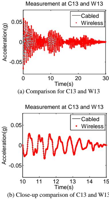
**Figure 5** Comparison of acceleration time history plots between cabled and wireless system
