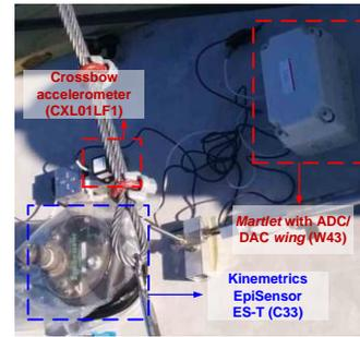
(a) Cabled and wireless accelerometer
