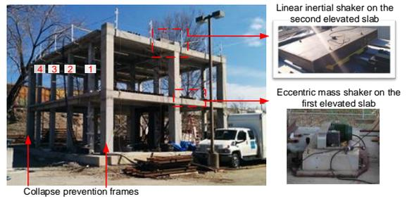
**Figure 1** Photo of test frames and two shakers on Frame 1 under test (viewing from southwest corner)
