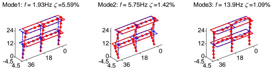
**Figure 6** First three identified mode shapes of Frame 1 (El Centro 1")
