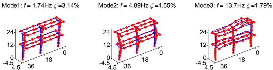
**Figure 7** First three identified mode shapes of Frame 1 (El Centro 4")
