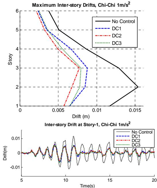
Fig. 4: Experimental Interstory Drift Results
