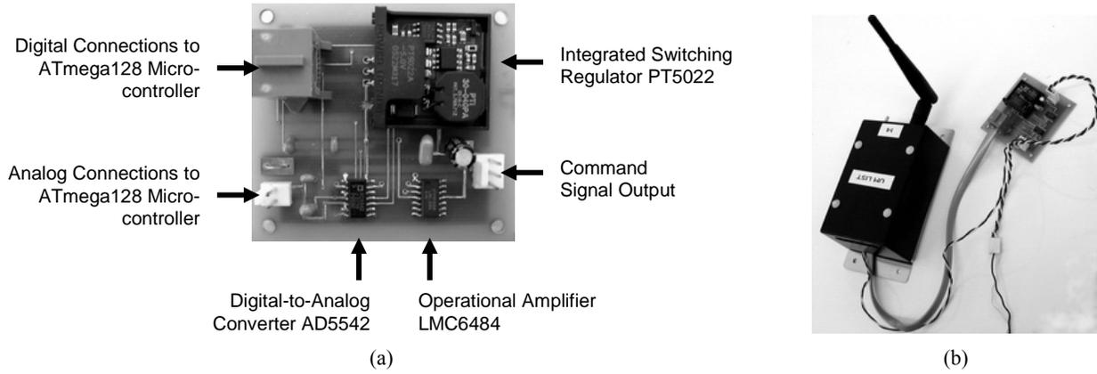
Figure 3. Pictures of the control signal module: (a) PCB board (5.5cm × 6.0 cm); (b) control signal module connected to wireless sensor
