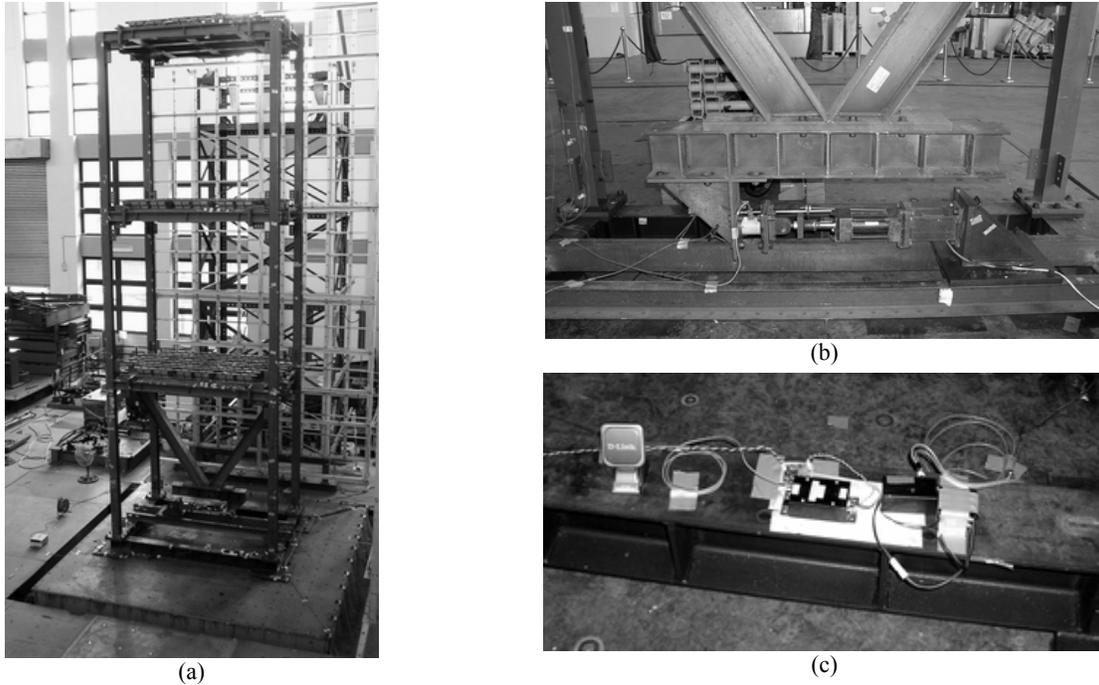
Figure 5. Laboratory setup: (a) the three-story test structure mounted on the shaking table; (b) the MR damper installed between the 1<sup>st</sup> floor and the base floor of the structure; (c) the wireless control unit commanding the MR damper.
