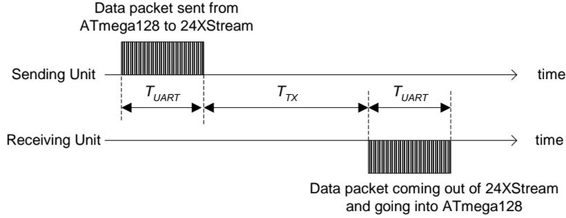
Figure 4. Communication latency of a single wireless transmission
