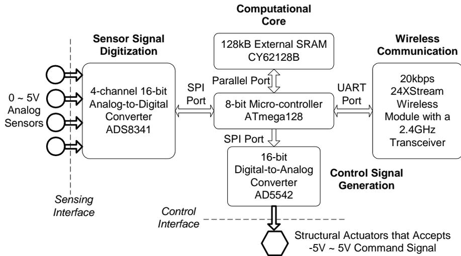
Figure 2. Hardware architecture of the wireless control unit
