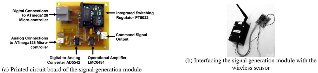
Fig. 5. Wireless sensing and actuation prototype unit.
