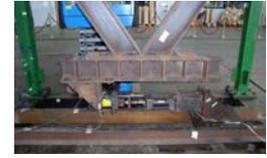
(c) MR damper installed between floors
