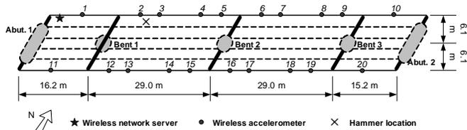
(a) Wireless accelerometer deployment for operating deflection shape analysis
