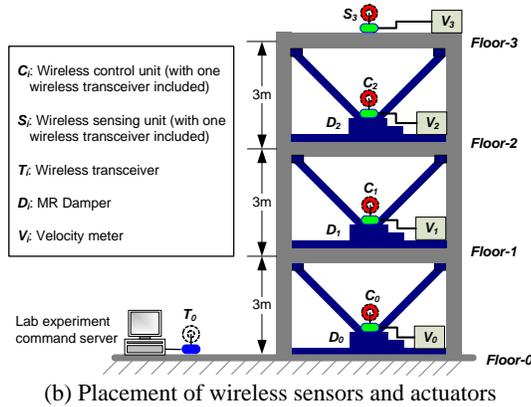
(b) Placement of wireless sensors and actuators
