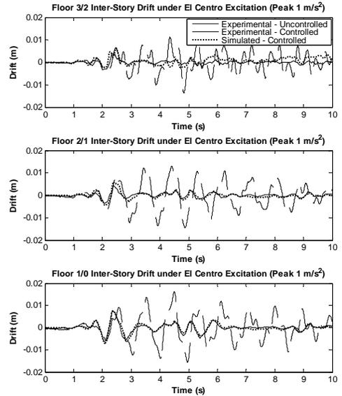
Fig. 7. Wireless control experimental results.
