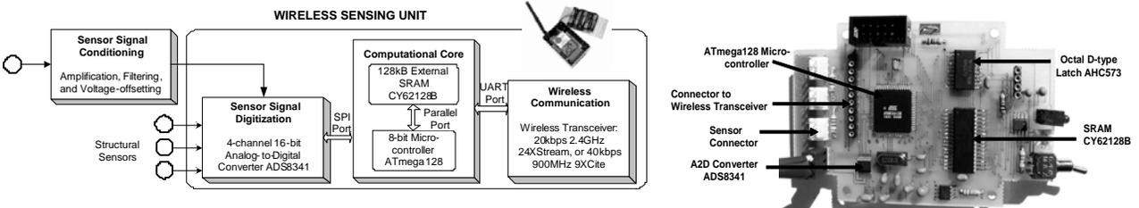
Fig. 1. Functional diagram detailing the hardware design of the wireless sensing unit.
