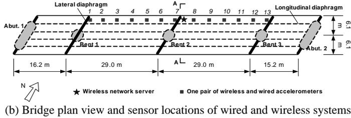
(b) Bridge plan view and sensor locations of wired and wireless systems
