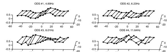
(b) Operating deflection shapes extracted from wireless sensor data
