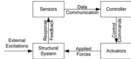
Fig. 4. Schematic of a structural control system [5].
