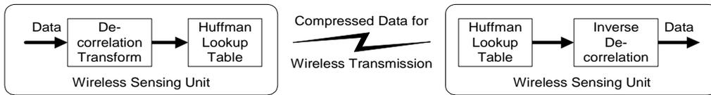
**Figure 5. Huffman Compression of Sensor Data using Wireless Sensing Units**
