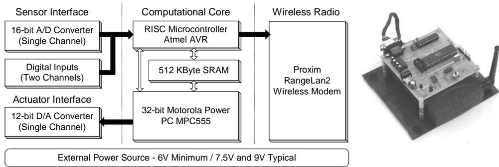
**Figure 1. Design of Prototype Wireless Sensing and Actuation Unit**
