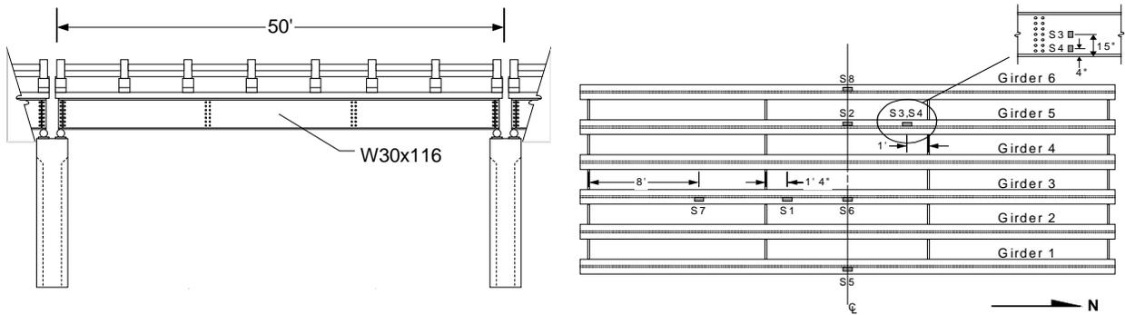
**Figure 3. Structural Details of the Alamosa Canyon Bridge**
