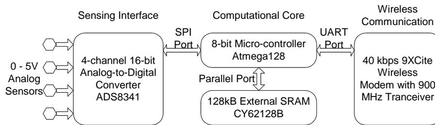
Figure 1 – Hardware functional diagram of the wireless sensing unit prototype
