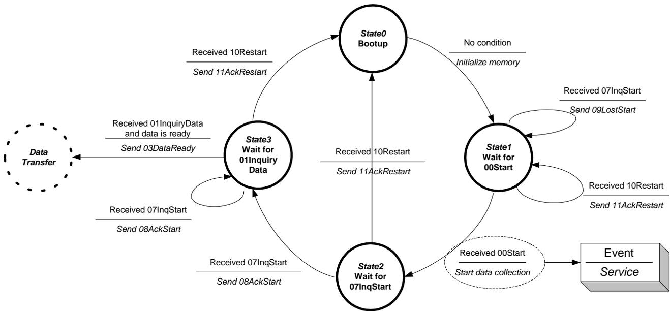
Figure 4 – Abridged communication state diagram for the wireless sensing unit
