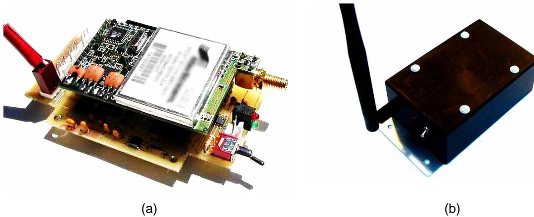
Figure 2 – Pictures of the wireless sensing unit prototype and the complete package
