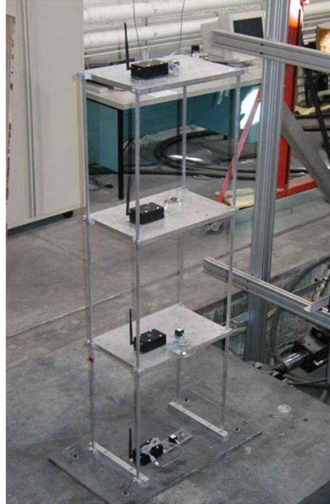
Figure 5 – Test structure for laboratory validation of the wireless monitoring system
