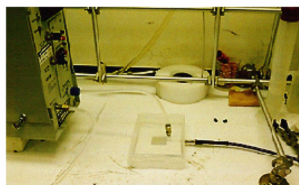
Fig. 2. Closed system measurement setup using a gas generator and ammonia permeation tubes. [3]
