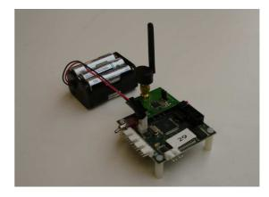
Figure 2 Narada wireless sensing and actuation node
