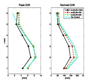
Figure 6 Peak and normed drift by floor due to the El Centro ground motion under MBC as the with diminishing initial wealth allocations
