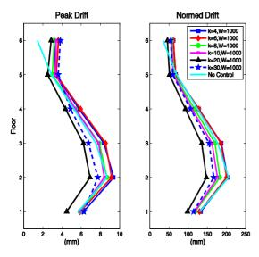
Figure 5 Peak and normed drift by floor due to the El Centro ground motion under MBC as the price to control force conversion factor increases
