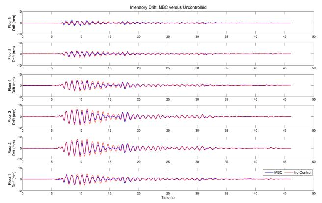
Figure 4 Time-history drift response of six-story to the scaled El Centro ground motion system under MBC, K = 20, initial wealth = 1000 for all floors
