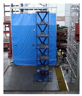
Figure 3 Six-story test structure mounted to the 25 m<sup>2</sup> shaking table at the National Center for Research on Earthquake Engineering (NCREE), Taipei, Taiwan
