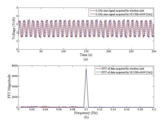
Figure 6. Wireless unit calibration using a standard sinusoidal signal generated by Agilent 33220A function generator: (a) Voltage data acquired by wireless unit and NI USB-6009 DAQ, (b) FFT magnitude
