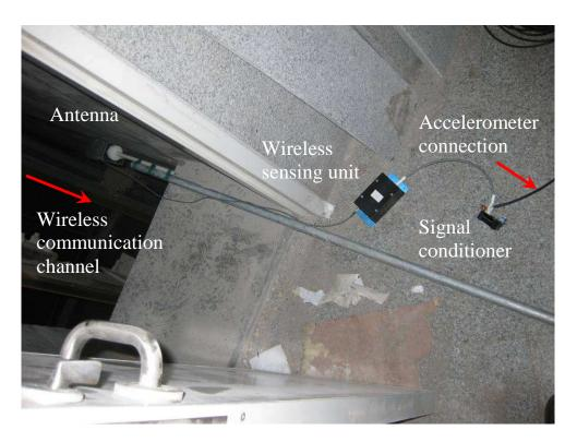
Figure 9. Experimental setup of the wireless sensing unit and the associated signal conditioning module inside the GTST
