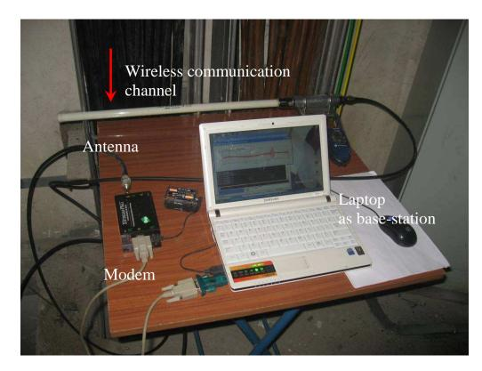
Figure 10. Experimental setup of the wireless base station at the site office on ground level
