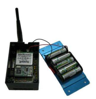
Figure 3. Wireless sensing prototype
