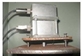
(b) Sensor setup for simultaneous measurements by wireless and wired systems
