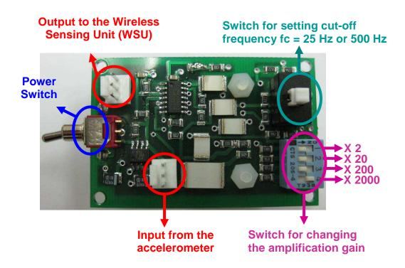
Figure 4. Low-noise high-gain (up to x2000) signal conditioning module
