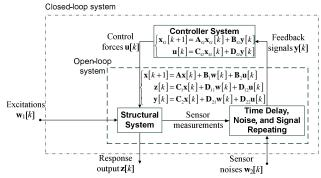
Fig. 1. Diagram of the closed-loop control system.
