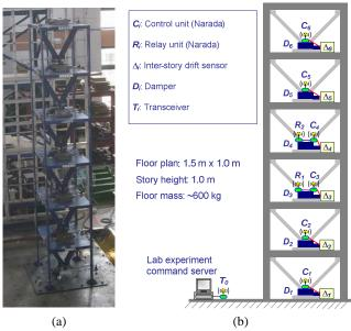
Fig. 2. Six-story structure for control experiments: (a) picture of the structure on the shake table; (b) schematic of the setup.
