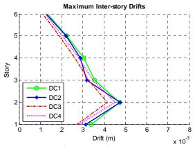
Fig. 5. Simulated peak inter-story drifts (with ideal actuators).
