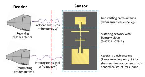
Fig. 1. Operation mechanism of a frequency doubling antenna sensor system
