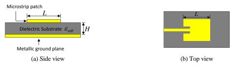
Fig. 2. Microstrip patch antenna
