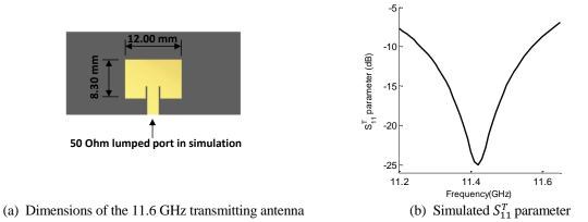
Fig. 4. Sensor-side transmitting antenna design
