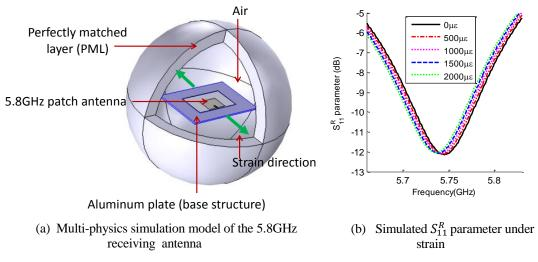
Fig. 6. Multi-physics modeling and simulation for the receiving (5.8GHz) patch antenna
