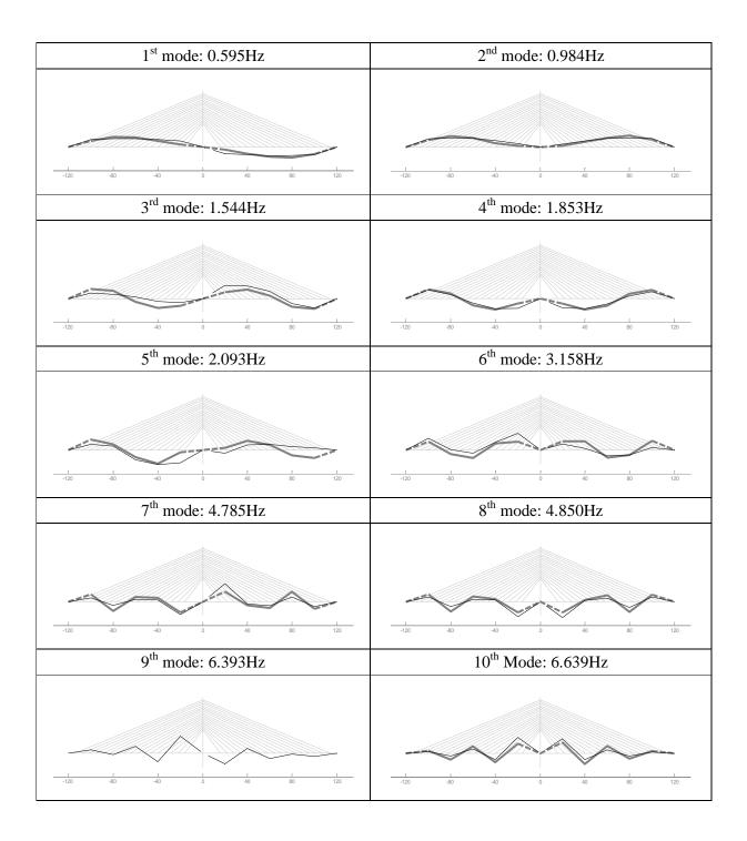
**Figure 8a:** Comparison of the identified bridge deck vertical mode shapes by using the reference-based stochastic subspace identification and frequency domain decomposition methods.
