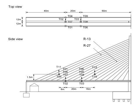
**Figure 1b:** Installation location of the wireless sensors during Test 3; velocity meters are installed to record the ambient response of the deck and cables simultaneously.
