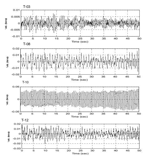
**Figure 7:** Recorded ambient vibration signals (velocity) at sensor location T03, T08, T10 and T12 (Fig.1b)( during Test-3.
