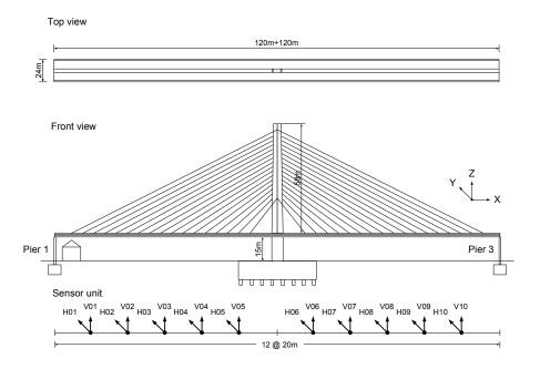
**Figure 1a:** Front view and top view of the Gi-Lu cable-stayed bridge. Locations of velocity meter-wireless sensor pairs installed (in vertical and transverse directions, for Test 1 and Test 2, respectively) along the bridge deck for the ambient vibration survey.
