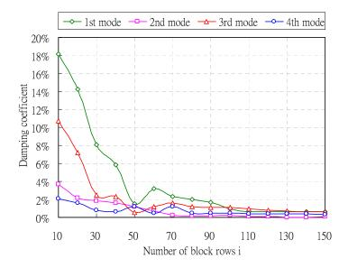
**Figure 6:** Relationship between the estimated modal parameters, natural frequency (a) and damping ratio (b), and the number of block rows "i". The sensitivity of the modal frequencies (a) and damping coefficients (b) can be identified with respect to "i".
