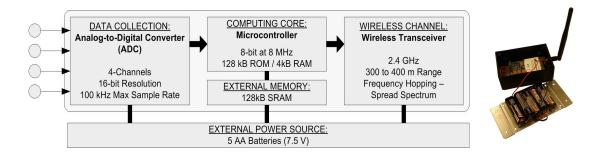
**Figure 2:** Overview of the hardware design of a wireless sensor prototype for structural monitoring applications [10].
