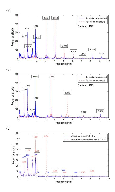
**Figure 9:** Fourier amplitude spectrum of cable vertical and horizontal vibration data (Fig. 9a for cable R-27 and Fig. 9b for cable R-13). The number in the box is the identified dominant frequency of cable. Comparison on the Fourier amplitude spectrum of cable vibration and deck vertical vibration is shown in Fig.9c.
