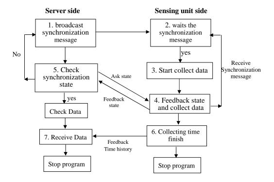
**Figure 3:** State diagram detailing time-synchronized communication between wireless sensing units and the data server.
