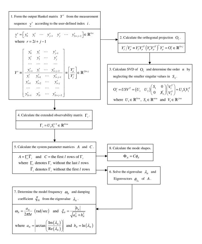
**Figure 4:** Flow chart of Stochastic Subspace Identification (SSI) technique.
