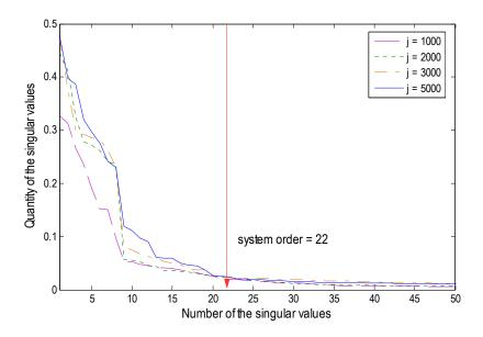
Figure 5: Plot of the singular value quantity as a function of the singular value index.
