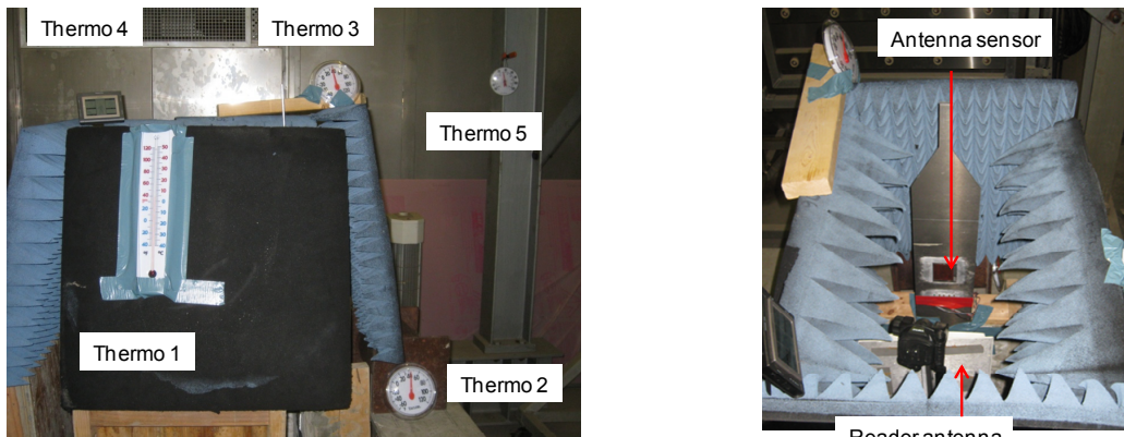
(a) Front view (test specimen is enclosed by foams) (b) Top view Fig. 6. Experimental setup for temperature chamber test
