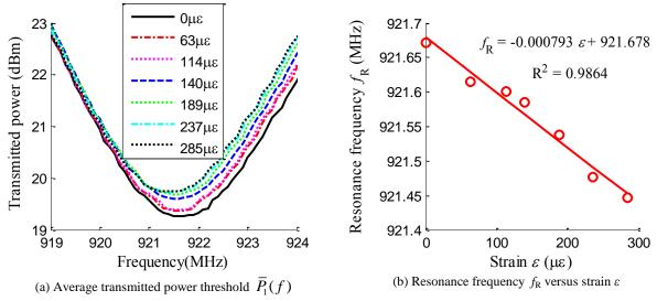
Fig. 9. Tensile testing results for the  $\sim$ 50  $\mu$ e/step loading case at 24 in. interrogation distance (Prototype A)
