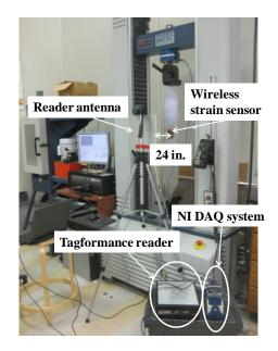
(a) Picture of the sensor instrumentation for wireless sensing experiments
