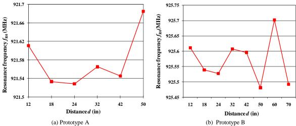
Fig. 13 Resonance frequency  $f_{R0}$  (at zero strain level) extracted from the transmitted power threshold plots in Fig. 12
