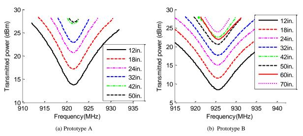
Fig. 12. Average transmitted power threshold plots (at zero strain level) for different interrogation distances
