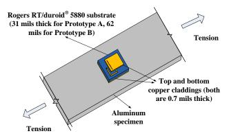
Fig. 4. RFID tag mounted at the center of an aluminum specimen (not to scale)
