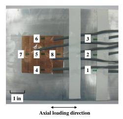
Fig. 5. Picture of the validation experiments for strain transfer
