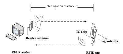
Fig. 1. Power transmission and backscattering in a passive RFID tag-reader system
