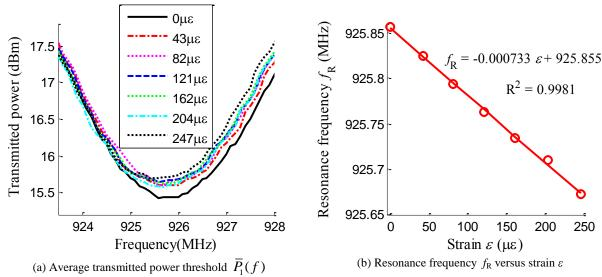
Fig. 10. Tensile testing results for the ~50 με/step loading case at 24 in. interrogation distance (Prototype B)
