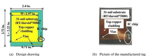
Fig. 2. RFID tag as wireless strain sensor (Prototype A)
