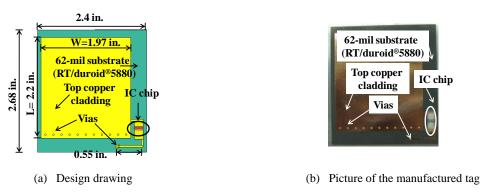
Fig. 3. RFID tag as wireless strain sensor (Prototype B)
