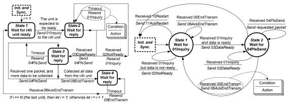
(a) State diagram of the server. (b) State diagram of a wireless sensing unit. Fig. 5. Communication state diagrams for wireless structural health monitoring.
