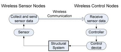
(a) Feedback control loop between the wireless sensing nodes and control nodes
