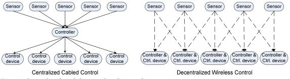
Fig. 10. Centralized and decentralized control systems.
