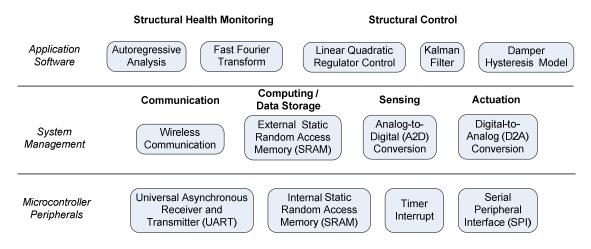
Fig. 2. Three-layer software architecture for the ATmega128 microcontroller in the wireless sensing and control unit.
