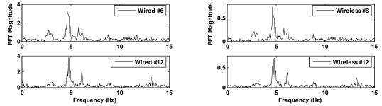
(b) Comparison between FFT to the wired data, as computed offline by a computer, and FFT to the wireless data, as computed online by the wireless sensing units Fig. 7. Comparison between wired and wireless data for the Voigt Bridge test.
