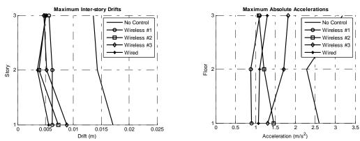
Fig. 17. Experimental results of different control schemes under 1940 El Centro NS earthquake excitation with peak ground accelerations (PGA) scaled to 1m/s<sup>2</sup>.
