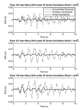
(b) Inter-story drifts of the structure with and without control.
