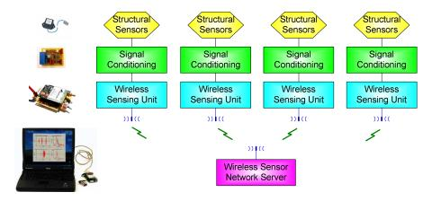
Fig. 4. An overview of the prototype wireless structural sensing system.
