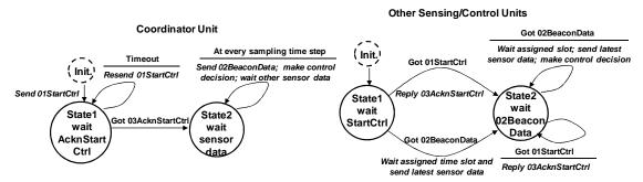
Fig. 12. Communication state diagram of a coordinator unit and other sensing/control units in one wireless subnet.
