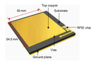
Fig. 1 RFID-based wireless antenna sensor
