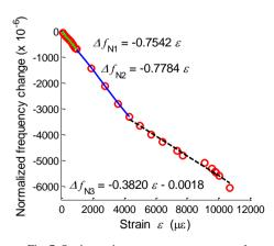
Fig. 7. Strain sensing measurement range results
