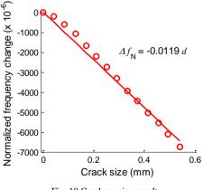
Fig. 10 Crack sensing results
