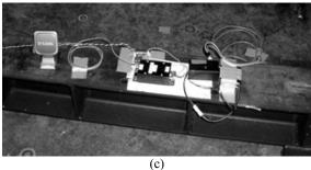
Figure 5. Laboratory setup: (a) the three-story test structure mounted on the shaking table; (b) the MR damper installed between the 1<sup>st</sup> floor and the base floor of the structure; (c) the wireless control unit commanding the MR damper.
