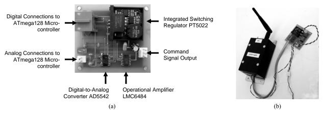
Figure 3. Pictures of the control signal module: (a) PCB board (5.5cm × 6.0 cm); (b) control signal module connected to wireless sensor
