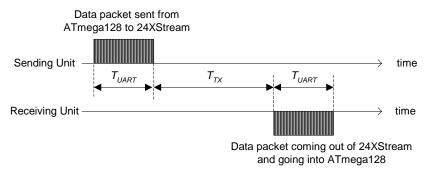
Figure 4. Communication latency of a single wireless transmission
