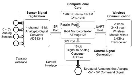
Figure 2. Hardware architecture of the wireless control unit
